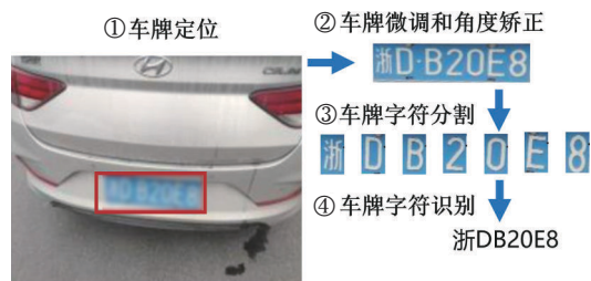
图7 车牌识别系统的识别流程 Figure 7 The recognition process of license plate recognition system
